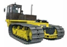
TM10.00B HST9 MT01 Crawler Tractor is a platform for special equipment. The machine is dedicated for transporting and power driving of snow tamper. In general, the complex is dedicated for constructing winter roads.
