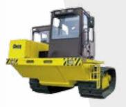
Besides, the crawler tractor TM10.00B HST9 MT01 can be used as a platform for drilling machines (USh2T type), manipulators with welding machines and other special implements; it is dedicated for pipeline construction and transportation of cargo or passenger (berthing) hodies
